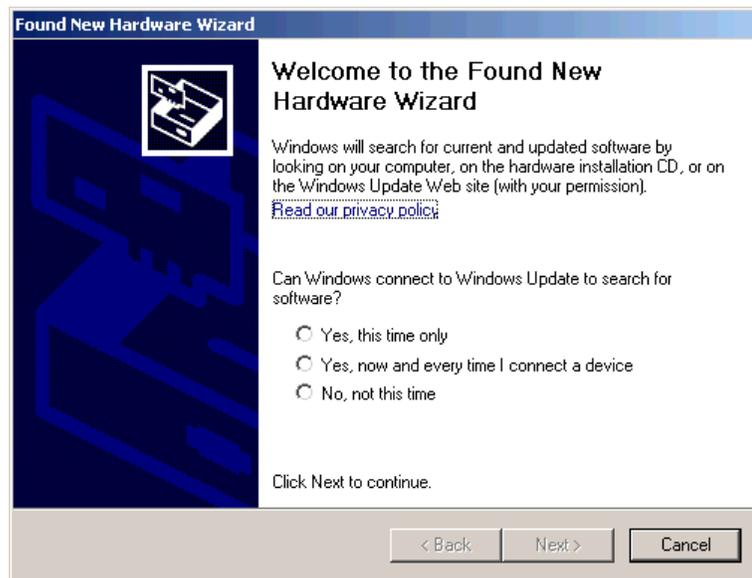
**TIP** If the software for the USB driver is not found and the installation is canceled, verify that you have installed RSLinx Classic software, version 2.59 or later.
